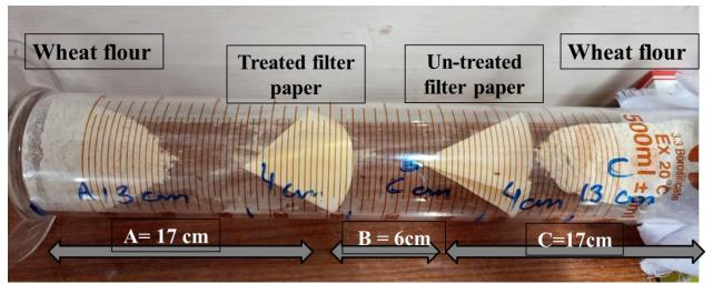
**Fig. 1.** Systematic diagram of cylinder trap for evaluating repellent efficacy of medicinal oils against *Triobleum castaneum*.
